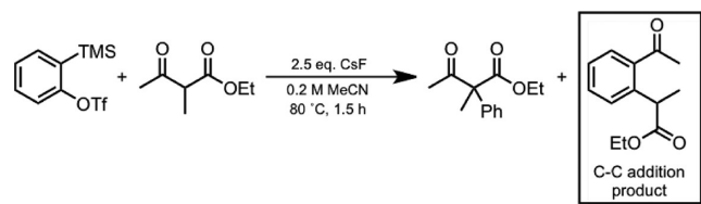
Scheme 1. Acyl-Alkylation of Benzyne into a β-Ketoester
